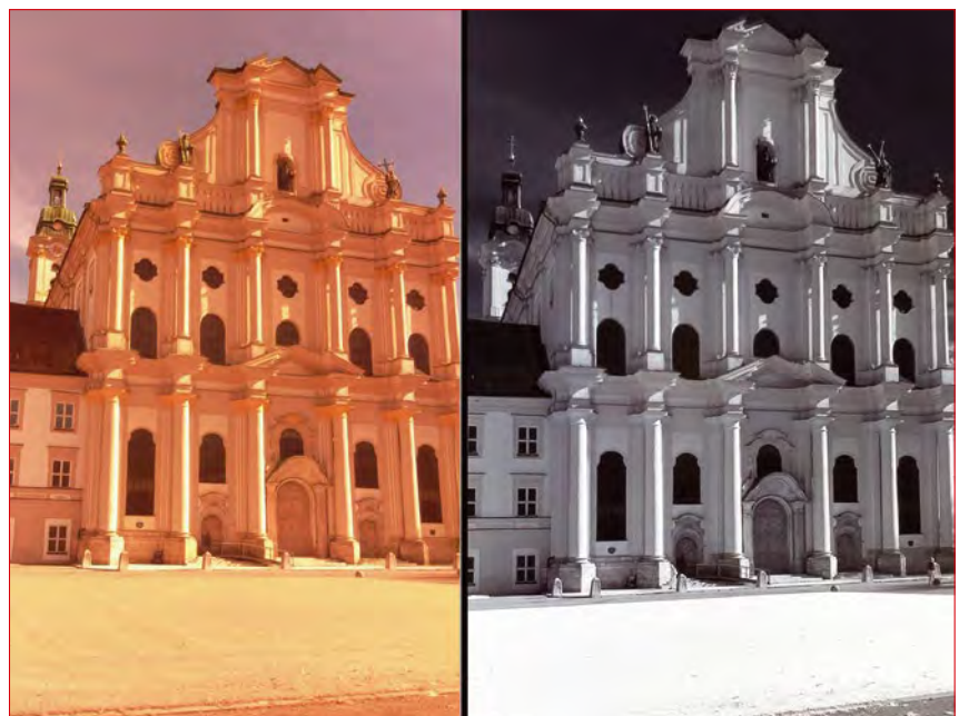
Figure 5: The photograph has far too many red tones (left) because the NoIR module lacks a band elimination filter. A 720nm filter blocks the normal light (right), so the camera captures only the infrared range.
