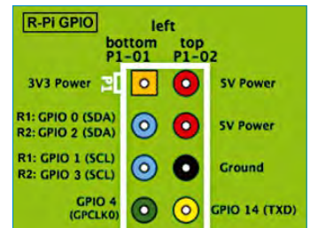
Figure 3: Pin changes from Rev 1 to Rev 2. (eLinux.com, CC BY-SA 3.0)
