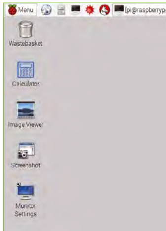
Figure 4: You can add icons to the desktop using Copy and Paste. Notice the little arrow at the top left of the Monitor Settings icon, indicating it is a link.
