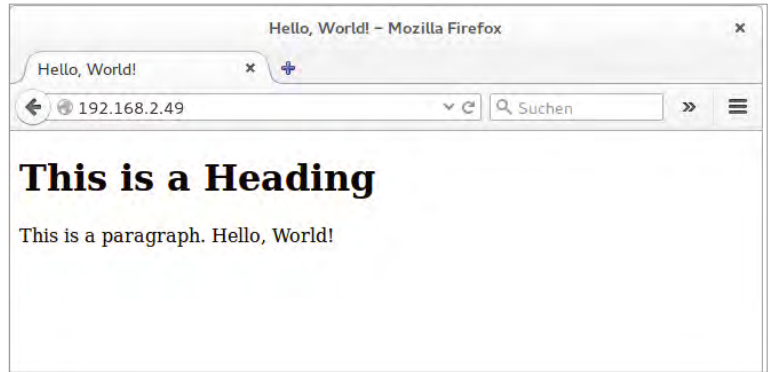
FIGURE 8: HTML describes the structure of a document. The code in Listing 1 produces this simple web page.
