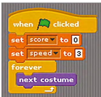
FIGURE 3: A stage script to initialize some game variables and to animate the backgrounds.
